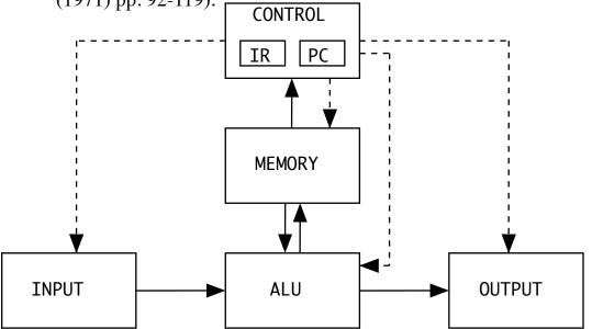
Solid lines = flow of data Dashed lines = flow of control
